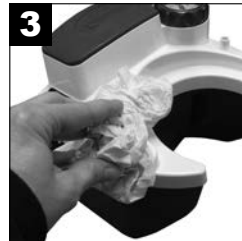
3 Wipe the housing with a clean cloth and any commercial (bacterial-germicidal) disinfectant.
